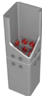
Field-Bolted HSS Splice
